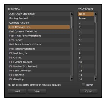
Select the desired MIDI controller number or, if you already have a hardware MIDI controller hooked up, move that controller for Jamstix to learn the controller. You can use the **Invert** switch to flip the control range so that low controller values yield high function values.
