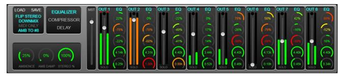
Jamstix provides 8 stereo audio outputs. Each channel can be toggled on and off via its label. There is a volume slider and associated LED level meter including a small red LED that signals brick wall limiter activity. Below the slider is a standard SOLO toggle button.
