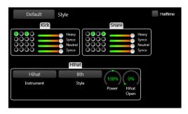
The grids work like this: every 'heavy' weight tick triggers a new column. So reading columns from left->right/top->down is like going through the bar sequentially in 16th notes. Click on a cell to add a hit. You can also right-click/hold/slide up-down on a hit to adjust velocity. The sliders to the right control the probability that any hit in that row will actually sound (great to create variability).
