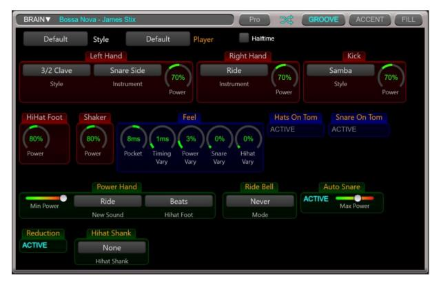
This is the heart of the Jamstix rhythm generation. The brain gives you access to the style and drummer of the current part. Both aspects are mixed into a list of control elements that apply to them. These items change from style to style and drummer to drummer. Style elements have a white frame while drummer elements have an orange frame.
