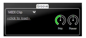
The groove importer is the focus of the 'Import' style but can also be added to any style via the 'Add' submenu of the brain menu. It allows you to load a MIDI drum pattern, Jamstix 1 rhythm or saved Jamstix 2/3 groove and have it fed into the composition process. If other groove elements are present, you will get a mix of the imported groove and them. Please watch the video 'Creating Your Own Base Groove' for more details.
