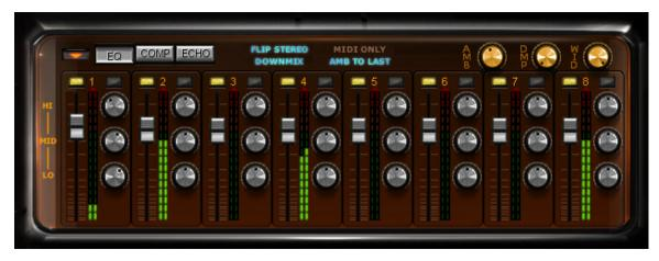
Jamstix provides 8 stereo audio outputs. Each channel strip has a yellow button to toggle the channel on and off. There is also a volume slider and associated LED level meter including a small red LED that signals brick wall limiter activity. Next to the toggle button is the number of the channel, which will display associated sounds of the current kit (roughly) in the status line when the mouse is moved over the channel number.
